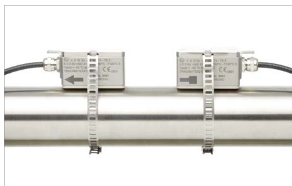
K1Ex transducers mounted using straps and clamps
